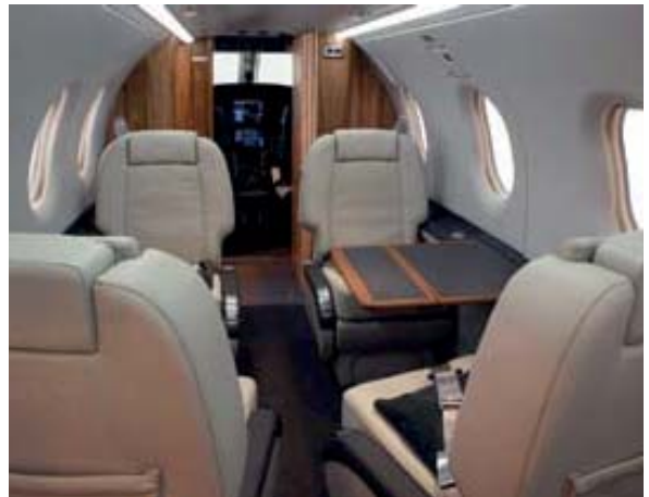
Interior trim and cockpit elements in PC-12 aircraft are bonded with our VOC-free contact adhesive.
